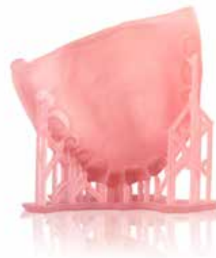
3D printed denture- image immediate after print process
