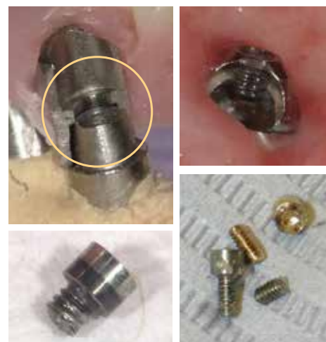
CURRENT COMPONENTS: Above illustrates fracture of the framework at the abutments interface. Universal conical connection with part of the screw lodged in the threaded portion of the abutment. Examples of fractured screws.
