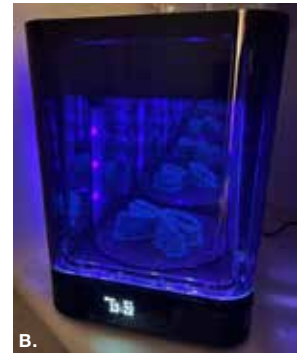
Figure 5. After surgical guides are printed, they are washed in the wash tank (A) with alcohol to remove excess resin prior to being cured (B)
