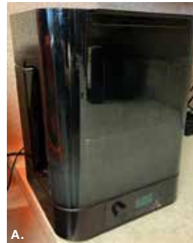
Figure 5. After surgical guides are printed, they are washed in the wash tank (A) with alcohol to remove excess resin prior to being cured (B)
